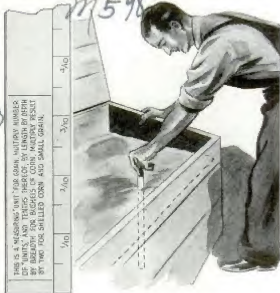
Special measuring stick, marked in tenths, reveals bushels in bin by multiplying the three dimensions
